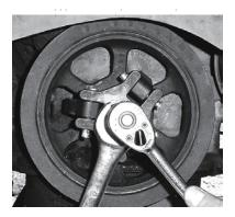
7. Remove the puller and balancer.
