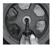
4. Select the rod from the kit that best matches your vehicle. The rod should bottom out in the hole.
