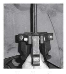
5. Place the rod through the puller and place the puller onto the balancer.
