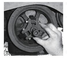
6. Feed the push bolt through the end of the puller and turn it clockwise until the balancer is freed from the engine block. This may require the use of a breaker bar or pneumatic tools, but if your vehicle has a crankshaft sensor take care not to thread the bolt deep enough to misalign or damage the sensor.
