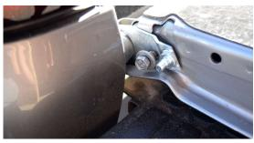
4. Apply the threadlocking fluid to the threads of the post. Install the post and the big washer where the cable bolt was previously. Tighten the fully threaded end of the post into the truck with a 13mm wrench.
