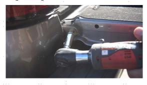
3. Detach the tailgate cable, and then remove the cable bold with a 13mm wrench.
