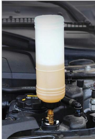
6. When refilling is complete, remove the bottle and reattach the reservoir cap.
