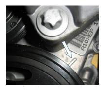
3. Locate and remove the blanking plug located at the front of the engine. This plug provides access to essential components for timing inspection and adjustment.
