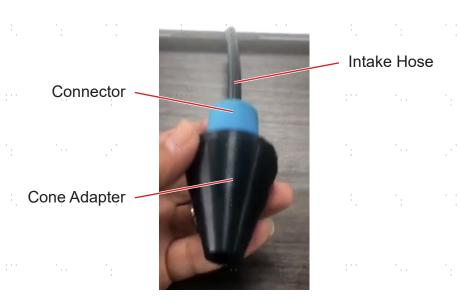
To use the large cone adapter (G), insert the smoke hose's nozzle into its intake hose underneath its curved surface and attach its vertex to the port. You can also remove its intake hose and then use the cone adapter base in the fashion above.
