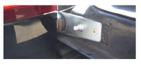
5. Hold the top mount plate in place vertically and use the cable bolt removed in Step 6 to install the top ball mount plate with a 13mm wrench. Ensure the plate does not rotate out of place when tightening.
