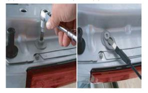
4. Insert the previously removed cable bolt through the hole of the upper ball mount plate and then use the torx wrench to reinstall the cable bolt with the mount plate back onto the vehicle.
