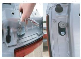
5. Use the provided mylar sheet to prevent any damage to your truck bed and tailgate during use. Cut the mylar sheet as needed with a pair of scissors. Apply the mylar to the truck bed and tailgate where components come in close contact during operation. The images below can be used as an example but the exact location should be adjusted according to your truck's specific requirements.
